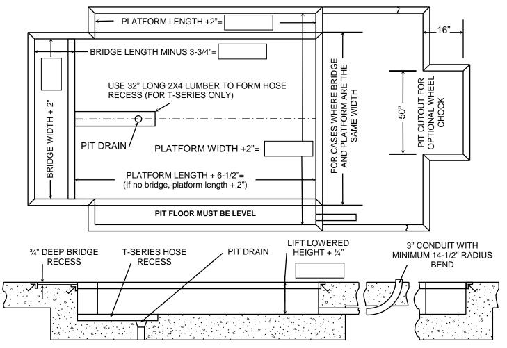
\*When mounting a "T-Series" lift on a pad it is necessary to supply a cutout in the concrete to allow passage of the hose under the base frame. T-Series lifts have no clearance between the platform and ground, any hose run through or over the base frame will be damaged when the platform is lowered.
